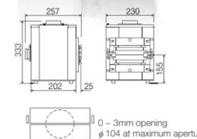
**Direct-viewing type** ▶ Defects and dust as small as 20 microns can be clearly viewed by placing a glass plate, etc., against the slit and introducing light through the edge.
