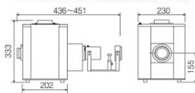
**Imaging type** ▶ Device is especially made for visually inspecting glass, lenses, and film, and for checking for scratches and bubble striae in permeable resins.
