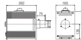
**Projection type** [High-collimation type] ▶ Device is especially made for visually inspecting glass, lenses, and film, and for checking for scratches and bubble striae in permeable resins.
