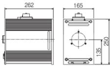
**Projection type** [High-intensity type] ▶ Device is especially made for visually inspecting glass, lenses, and film, and for checking for scratches and bubble striae in permeable resins.
